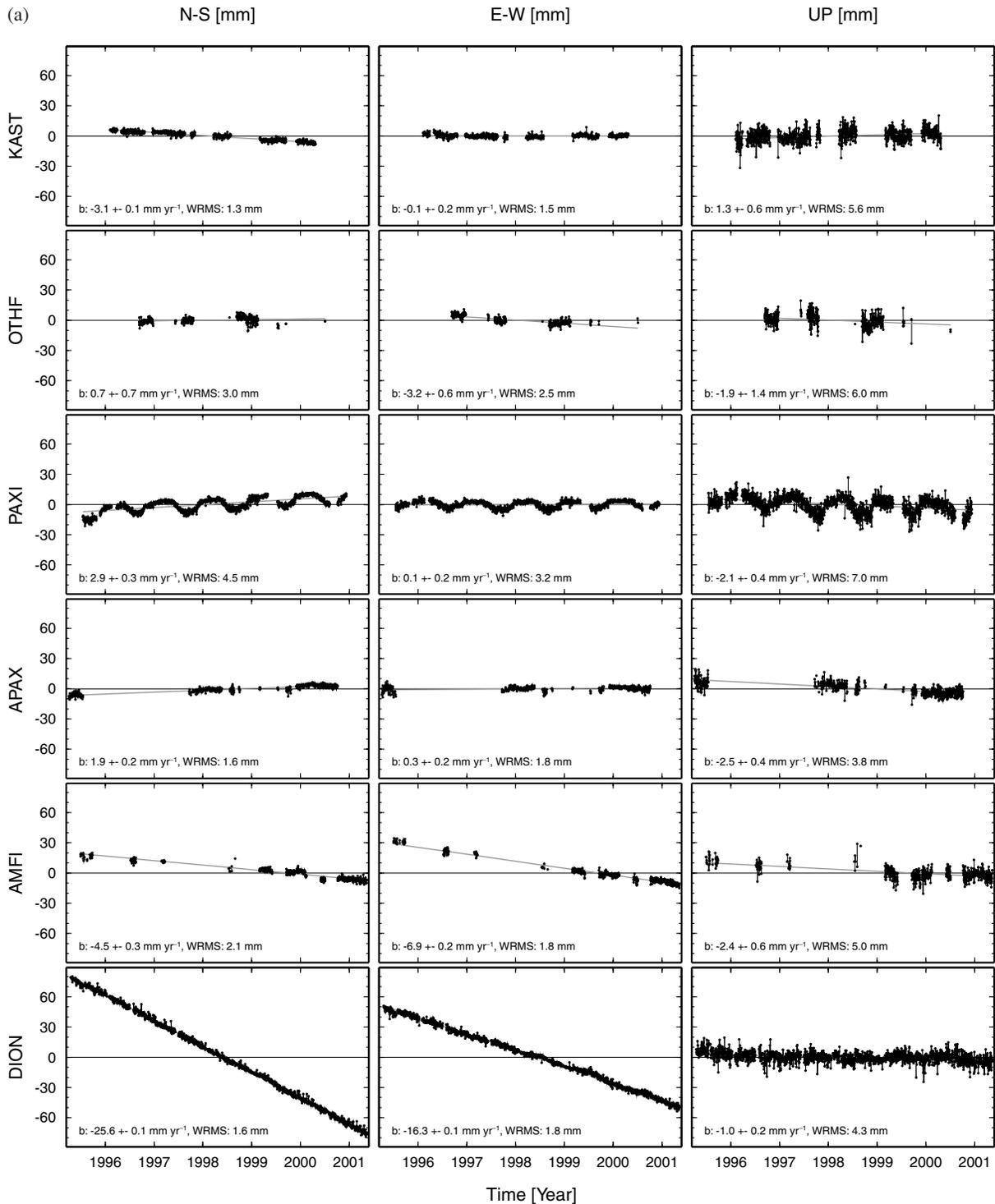
**Figure 5.** Common-mode filtered time-series of daily coordinates relative to Eurasia. ‘b’: velocity, calculated by weighted linear regression, formal error scaled by 4 (see chapter 4); b1: before, b2 after the Strofades earthquake. ‘WRMS’: weighted rms of daily coordinates. The grey lines represent the weighted linear fit.
