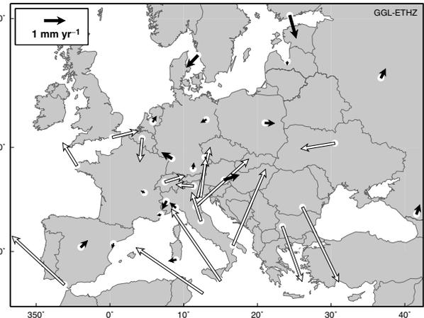
**Figure 2.** Velocity residuals with reference to the rotation of Eurasia (rotation parameters see chapter 3). Black arrows: velocities of sites which were included in the final pole estimation, white arrows: velocities of sites that were excluded during the iterations.
