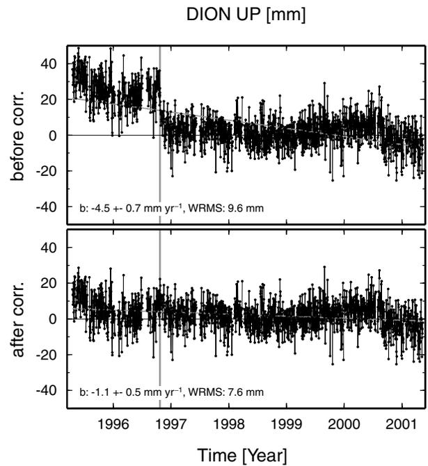
**Figure 4.** Correction of unknown variation of the phase centre offset due to an antenna change for the up-component of DION. Time-series before and after the correction (step 3). The vertical grey line marks the time of the antenna change. 'b': velocity, calculated by weighted linear regression, formal error scaled by 4 (see chapter 4); 'WRMS': weighted rms of daily coordinates.
