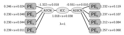
Figure 14: LSLA dynamic energy model inferred from energy measurements with computational quanta in ns, communication quanta in Bytes, and energy data vector d in nJ.  $PE_{1-4}$  are Cortex-A7 cores and  $PE_{5-8}$  are Cortex-A15 cores.
