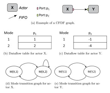
Figure 3: Dataflow attributes of an example CFDF graph.
