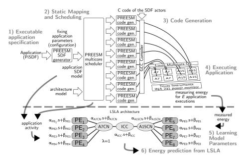
Figure 10: Experimental setup for inferring the LSLA execution energy model of a Samsung Exynos 5422 MPSoC.
