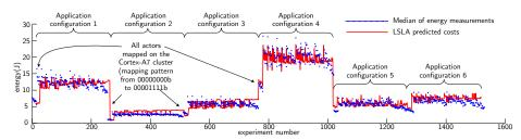
Figure 15: Comparing the LSLA predicted cost and the median of the corresponding energy measurements.
