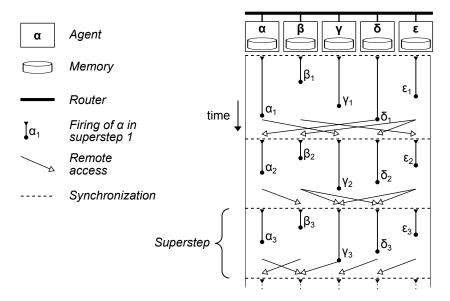
Figure 4: Example of a BSP Representation.
