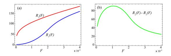
FIG. 17. a) Evolution as a function of F of the roots  $R_1$  and  $R_2$  of E(R) given by Eq. (24). b) Evolution of  $R_2 - R_1$  as a function of F. The parameters of the pulse are  $T_{\rm ru} = 15$  ps,  $T_{\rm p} = 70$  ps and  $T_{\rm rd} = 15$  ps.
