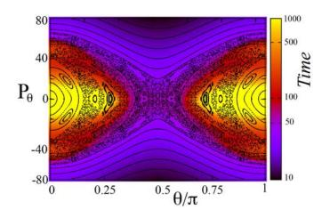
FIG. 8. First recurrence time (in ps) in the Poincaré section ( $P_R = 0, \dot{P}_R < 0$ ) in the plane ( $\theta, P_{\theta}$ ) for  $F = 1.5 \times 10^{-3}$  a.u. and energy  $E = -3.98 \times 10^{-4}$  a.u. The color axis has been saturated at 1000 ps for clarity. In the middle region, the recurrence time reaches above 1400 ps. Note that a logarithmic scale is used in the color code.
