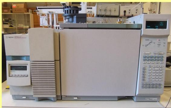
Agilent GC 6890 with 5973 N detector (GC-MS)
