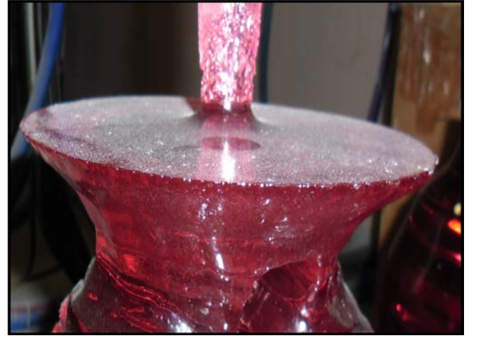
Fig. 8. Formation of a plateau and temporal concave shape of the crystal observed during the first stage of growth in crucibles of d = 30 \text{ cm} in diameter.
