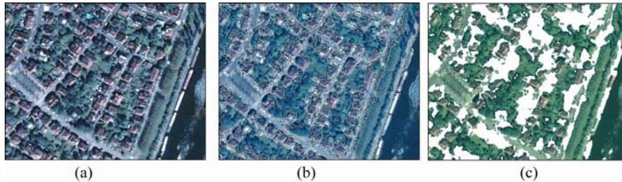
**Fig. 4.** a. Extract of the Quickbird image of the city of Strasbourg illustrating a typical individual house urban fabric. b. Segmented image. c. Recognized objects set (the unknown objects are highlighted in white).
