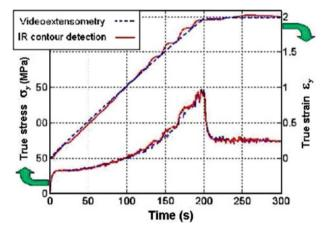
Fig. 3 Stress-Strain curve and longitudinal strain as produced by videoextensometry or IR contour detection
