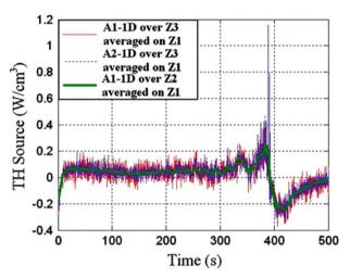
Fig. 8 Comparison between THS identified on  $Z_1$  with the 1-D algorithms applied on zones  $Z_2$  and  $Z_3$  ( $\dot{e}_{\gamma} = 0.005 \text{ s}^{-1}$ )
