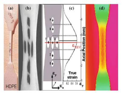
Fig. 1 Videoextensioneter system and infrared imaging: a deformed specimen, b snapshot of videotraction markers, c principle of videotraction longitudinal strain measurement on a REV, d temperature field for a given deformation with necking
