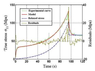
**Fig. 11** Experimental and theoretical fitted curves  $\sigma = f(t)$  for the tensile-relaxation test at  $\dot{\varepsilon}_1$
