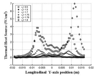
Fig. 10 Reconstructed THS profile at different strains for a tensile test at  $\dot{\varepsilon}_y = 0.01 \text{ s}^{-1}$
