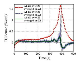
**Fig.** 7 Identification of 1D and 2D THS on zones  $Z_1$  and  $Z_3$  ( $\dot{\varepsilon}_v = 0.005 \text{ s}^{-1}$ )
