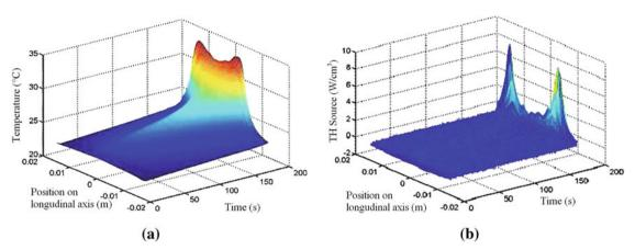
Fig. 9 Temperature and TH Source maps (test at  $\dot{\varepsilon}_{\nu} = 0.01 \text{ s}^{-1}$ ). a Temperature. b THS
