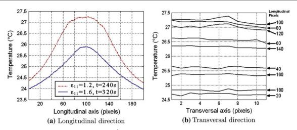
Fig. 5 Temperature profiles (test at  $\dot{\varepsilon}_y = 0.005 \text{ s}^{-1}$ ). a Longitudinal direction. b Transversal direction
