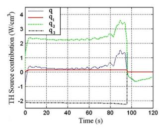
Fig. 13 Theoretical curve  $\dot{q} = f(t)$  for the tensile-relaxation test at  $\dot{e}_1$  and behavior of the thermomechanical components  $\dot{q}_1$ ,  $\dot{q}_2$  and  $\dot{q}_3$
