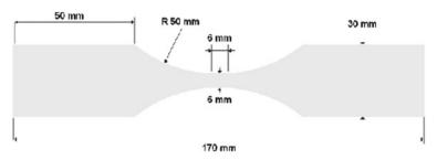
Fig. 2 Shape and dimensions of the specimen used for tensile test
