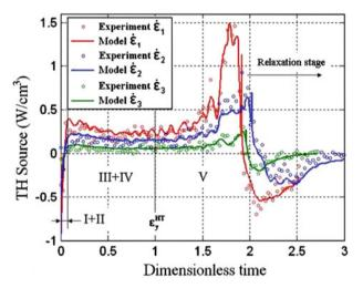
Fig. 12 Experimental and theoretical fitted curves q = f(t) for the tensile-relaxation test at three different strain rates
