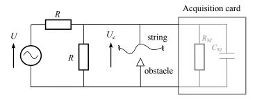
Figure 9: Electric scheme for contact detection.
