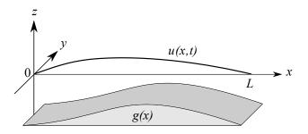
Figure 1: A string of length L vibrating against an obstacle q(x).
