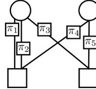
Fig. 1: The ‘vectorized’ protograph ldpc code generated by “copy-and-permute” operations. Each interleaver  $\pi_i |_{1 \leq i \leq 5}$  permutes the bundle of the  $N$  replicas of each edge.
