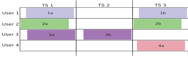
Fig. 1: A part of a frame (three time slots) with four users transmitting their packets to a destination D
