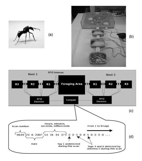
Fig. 1: The RFID environment: (a) Ant with RFID tag. (b) Snapshot of a part of the ant nest. One can appreciate the three rooms of the old nest and the foraging area.(c) The RFID experimental device. (d) Example of a recorded scan in the data file
