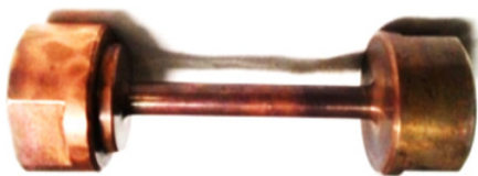
Figure 4. CuBe pressure cell (sample holder).
