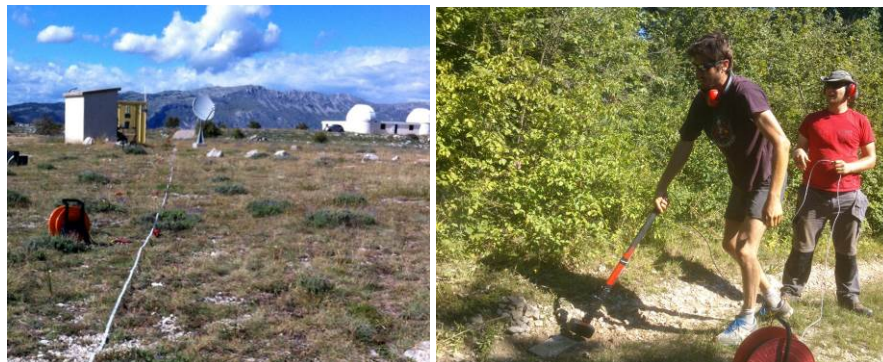
Figure 2 – Left: MASW line near the CALF station. Right: MASW acquisition (4 kg hammer source) near the OGCH station.
