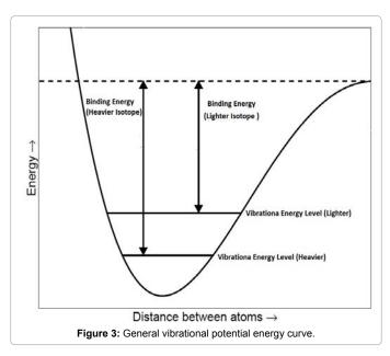
potential energy curve remains same (Figure 3). Furthermore, the vibration energy level of a bond in a molecule can be represented by following equation [26].
