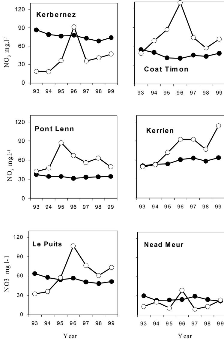
Fig 5. Variations of the mean annual nitrate concentration ( $\text{mg NO}_3\text{l}^{-1}$ ), in streamwater (black symbols) and in the drainage water as calculated from the 'corrected budget' (white symbols) for the six catchments.
