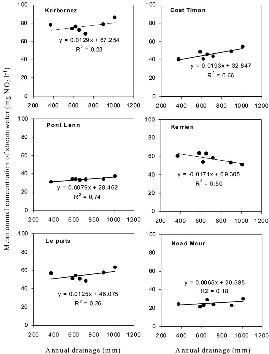
Fig 2. Nitrate concentration in streamwater (mg NO<sub>3</sub> l<sup>-1</sup>) vs mean annual amount of drainage water (mm) for the six catchments.
