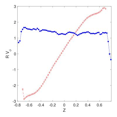
**Figure 9.** Profiles of angular momentum  $RV_{\phi}$  as a function of Z in the von Karman laboratory experiment. Blue symbols with line: in the *bifurcated* state with higher dissipation. Red line with symbols: in the symmetric state.
