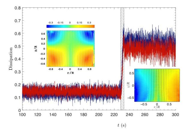
**Figure 3.** Spontaneous bifurcation in the von Karman flow: the flow, initially started in a symmetrical state, bifurcates after a certain time toward a bifurcated state, that produces a 4 times larger dissipation [5].
