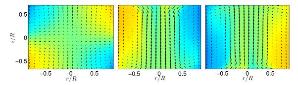
**Figure 2.** The 3 stationary states of the von Karman flow: left: The symmetric state. Middle and right: the two bifurcated states, that are symmetric to each other with respect to a  $\pi$ -rotation along an axis going through the rotation axis [5,6].
