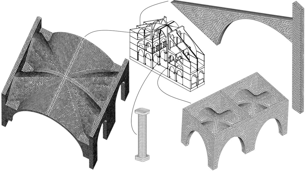
Figure 7: Details of the mesh used for the finite element analyses.
