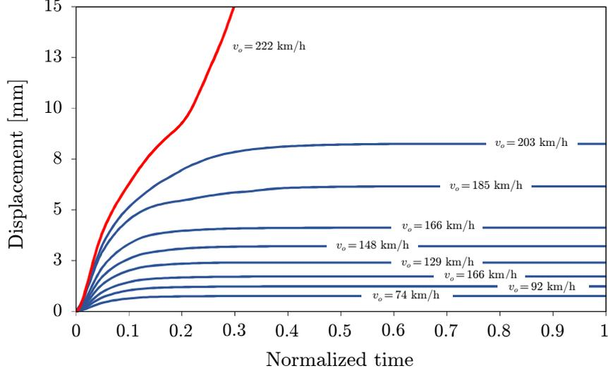
Figure 14: Diagrams time-displacement for various wind speeds  $v_0$ .
