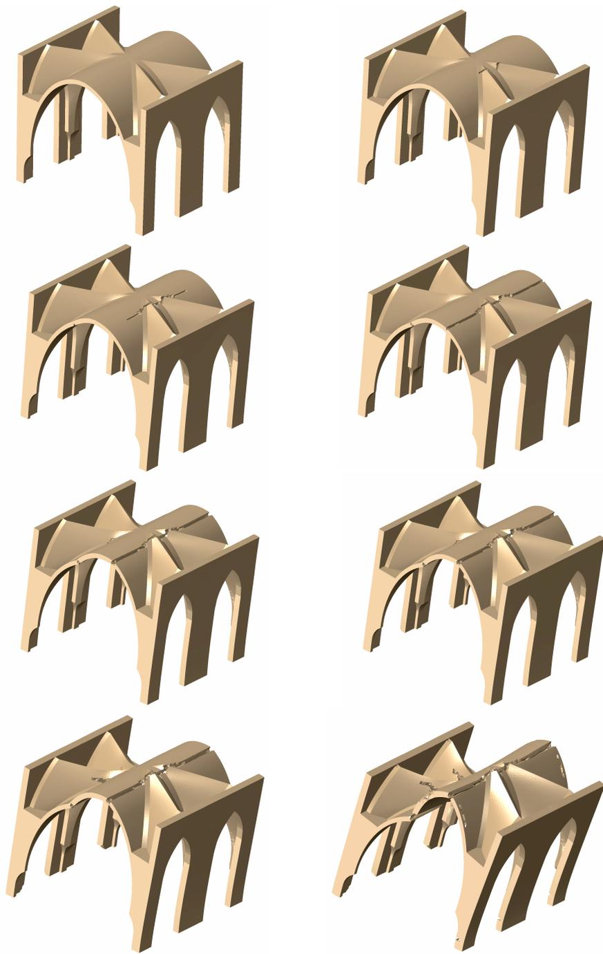
Figure 20: Progressive failure of the high sexpartite vault
