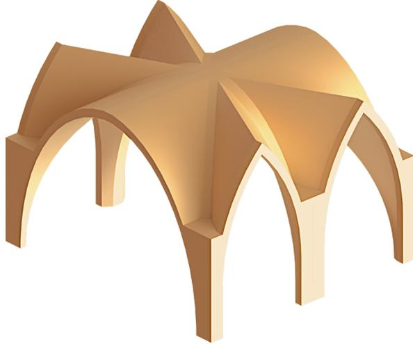
Figure 5: The numerical model of Notre Dame of Paris: the sexpartite vault.
