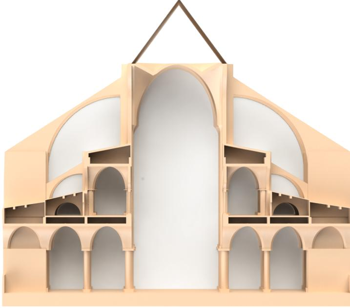
Figure 4: The numerical model of Notre Dame of Paris: transversal section.
