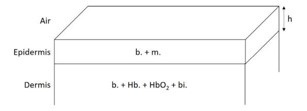
Figure 3. Skin model with two layers. Epidermis is composed of baseline (b.) and melanin (m.) and has a thickness h. Dermis is composed of baseline (b.), deoxy-hemoglobin (Hb.), oxy-hemoglobin (HbO<sub>2</sub>) and bilirubin (b.). Its thickness is assumed to be infinite.
