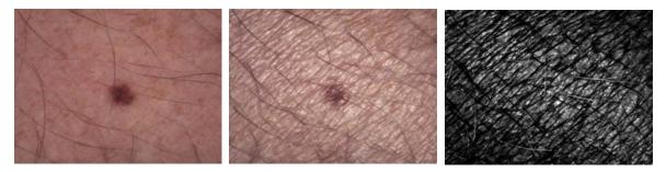
Figure 2 – Same skin area observed by the hyperspectral imaging system in cross-polarization mode (left) or parallel-polarization mode (center); subtracting the two images yields the gloss image displayed on the right. Here, hyperspectral images are converted into RGB color images.
