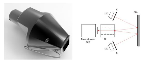
Figure 1 – SpectraCam (left) and its schematic (right). Light emitted by LEDs is transmitted through the polarizers (**P**.) and reflected by the skin. A tunable filter (**TF**) let pass a specific wavelength and is used as analyzer. The resulting image is captured by a monochromatic camera.
