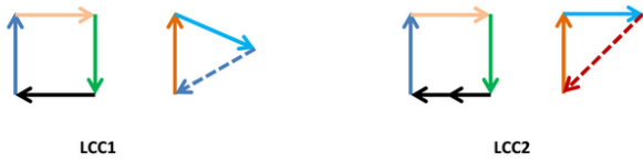
Figure 3: Example of association between darts: darts with the same color are associated. Two black darts of LCC2 are associated with only one dart of LCC1. Dotted darts are not associated because 3D points on their origins are different.
