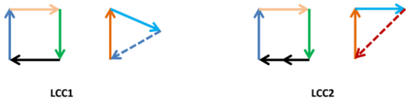
Figure 3: Example of association between darts: darts with the same color are associated. Two black darts of LCC2 are associated with only one dart of LCC1. Dotted darts are not associated because 3D points on their origins are different.
