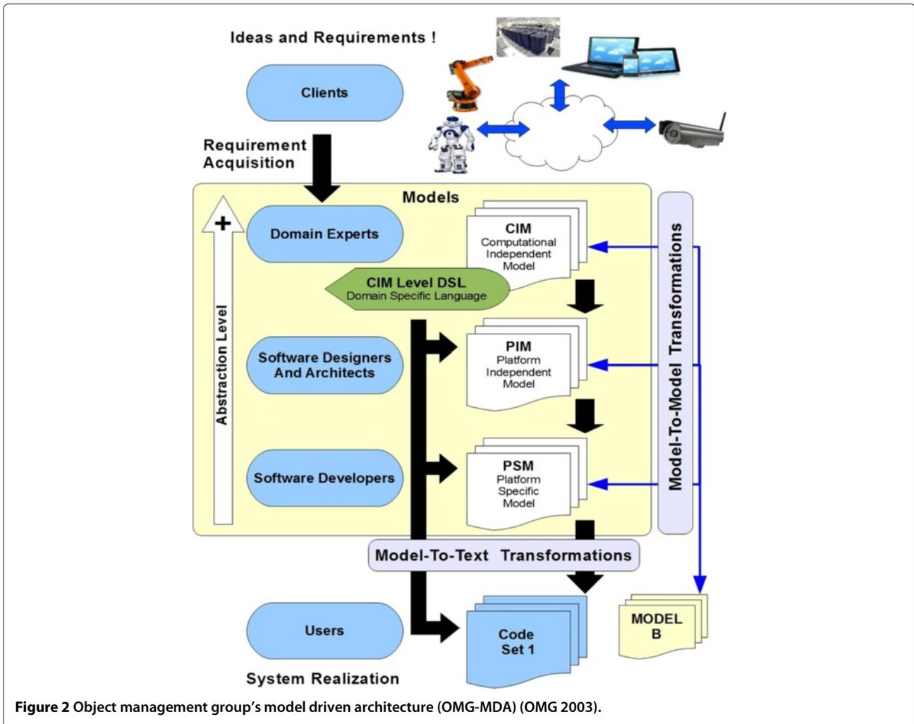
Figure 2 Object management group’s model driven architecture (OMG-MDA) (OMG 2003).
