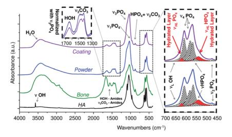
Fig. 2. FTIR of BNAc coating obtained by cold spray, BNAc powder, bone,  $^{[55]}$  and stoichiometric HA; lateral insert: deconvolution from 450 to 700 cm $^{-1}$  and front insert: normalized view (height of  $v_3PO_4$ ) from 1 300 to 1750 cm $^{-1}$ .
