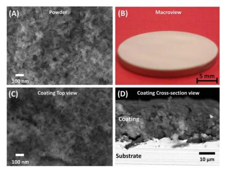
Fig. 3. (A) SEM micrograph of powder, (B) coated material macroview, (C) SEM micrograph of coated material (top view), and (D) SEM micrograph of cross-section of coated material.
