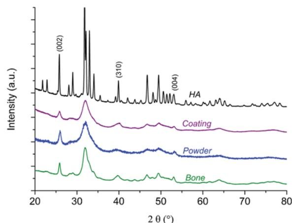
Fig. 1. XRD pattern of BNAC coating obtained by cold spray, BNAC powder, human bone,<sup>[54]</sup> and stoichiometric HA.
