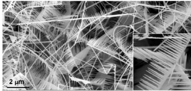
FIG. 72. SEM image of nanocombs consisting of nanoribbons grown along the [2\bar{1}\bar{1}0] direction with \pm(0001) side surfaces, on which NWs are more slowly formed along the [0001] direction while no growth occurs along the [000\bar{1}] direction. Reprinted with permission from Ref. 583. Copyright 2003 American Physical Society.
