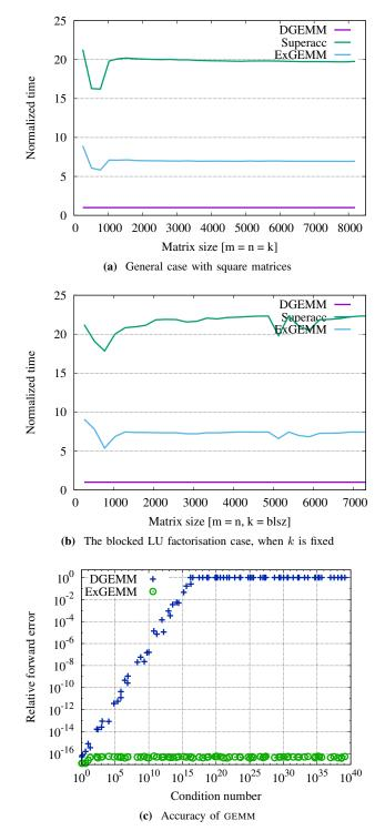
Figure 4: Performance and accuracy results of GEMM; *blsz* stands for the block size, which was set to 256.
