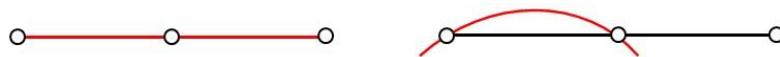
Figure 6: the two cases of multiple cancelations of the level sets along a three node edge which are authorized.
