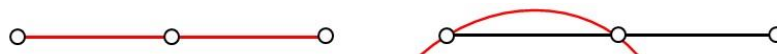
Figure 6: the two cases of multiple cancelations of the level sets along a three node edge which are authorized.
