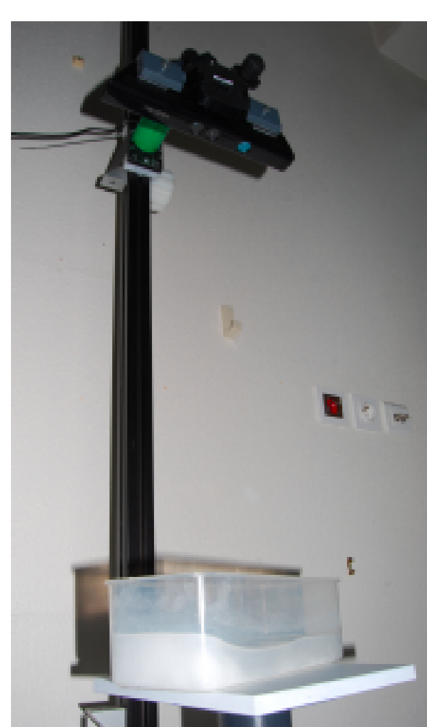
Figure: Experiment configuration with the depth sensor (Kinect sensor)
