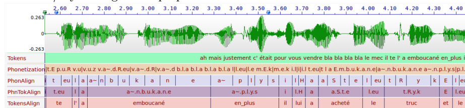
Fig. 3. SPPAS output example from CID (spontaneous speech). The regional word “emboucané” was missing in the dictionary and automatically rightly phonetized /ã b u k a n e/ by the algorithm proposed in section 3.4.
