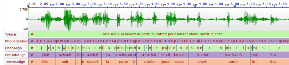
Fig. 2. SPPAS output example from AixOx (read speech). The truncated word “chort-” was missing in the dictionary and automatically rightly phonetized /ʃ o ʁ t/ by the algorithm proposed in section 3.4.
