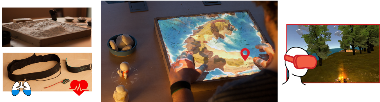
Figure 1. Inner Garden: A sandbox (up left) is connected to physiological sensors (bottom left) to create a mindful interactive experience where the user can shape her own world that evolves according to her breathing and heart rate (center). The user can then decide to be immersed inside this world thanks to a Head Mounted Display (right) for a moment of solitude and meditation.
