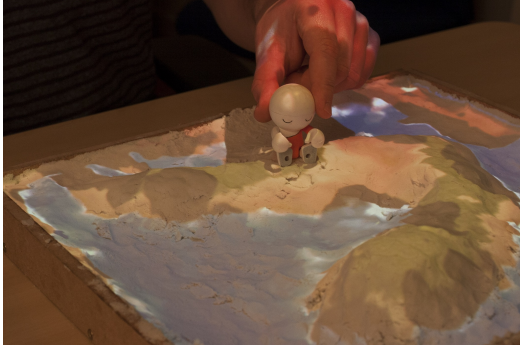
Figure 2. A physical avatar allows the user to choose the location where he or she wants to be immersed in his or her mini-world.
