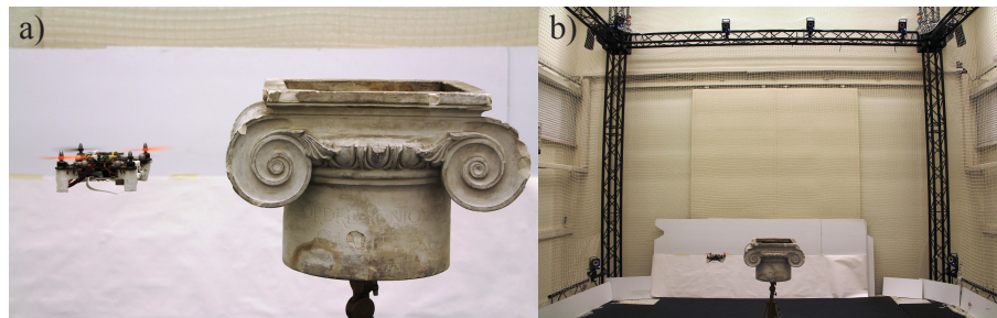
Figure 1. (a) The X4-MaG quadrotor equipped with an embedded Raspberry Camera weighs 367 grams and can fly autonomously for 10 min. It can fly closer to the artifact (here, a capital) to capture more details without endangering the artifact itself because of its small size and low weight. (b) The flying test arena in Marseilles with its 17 Vicon cameras can be used to control the quadrotor's trajectory around the artifact. The ground-truth Vicon system provides the position of the quadrotor used for monitoring purposes, which is necessary to control in a closed loop.
