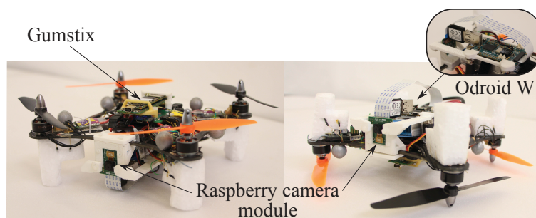
Figure 2. The X4-MaG robot is fully controlled via the Linux-based controller embedded onboard the Gumstix Overo. The image acquisition is performed with an Odroid W board and its small 5-Mpx Raspberry Camera Module.
