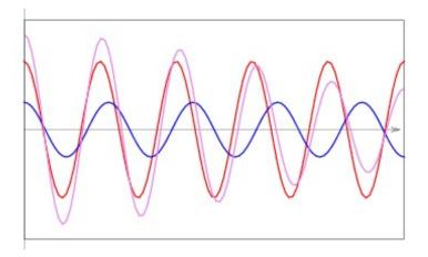
Figure 5: Addition of different frequency sinusoids (red and blue), before beats.
