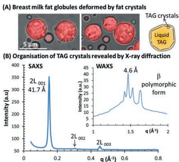
► Figure 1: Fat crystals formed upon storage of breast milk in the fridge. (A) Microscopy images showing the deformation of breast milk fat globules induced by crystals of triacylglycerols (TAG), and schematic representation. (B) Structural analysis of the TAG crystals performed by synchrotron radiation X-ray diffraction at small (SAXS) and wide (WAXS) angles at 4°C.
