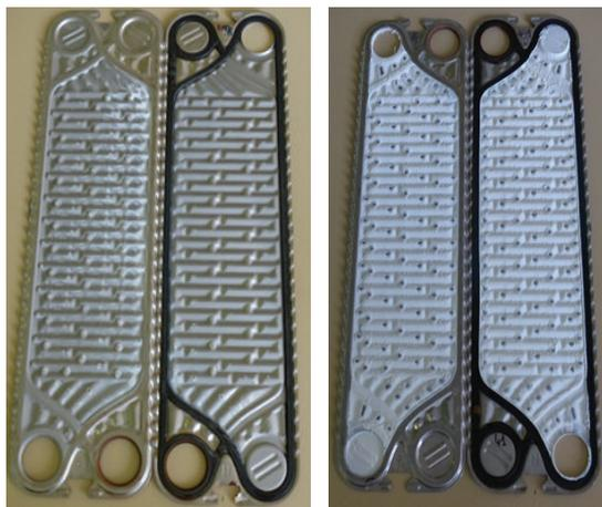
FIGURE 6: Pictures of the deposit collected on heat exchanger surface in the second and last channels of the PHE.
