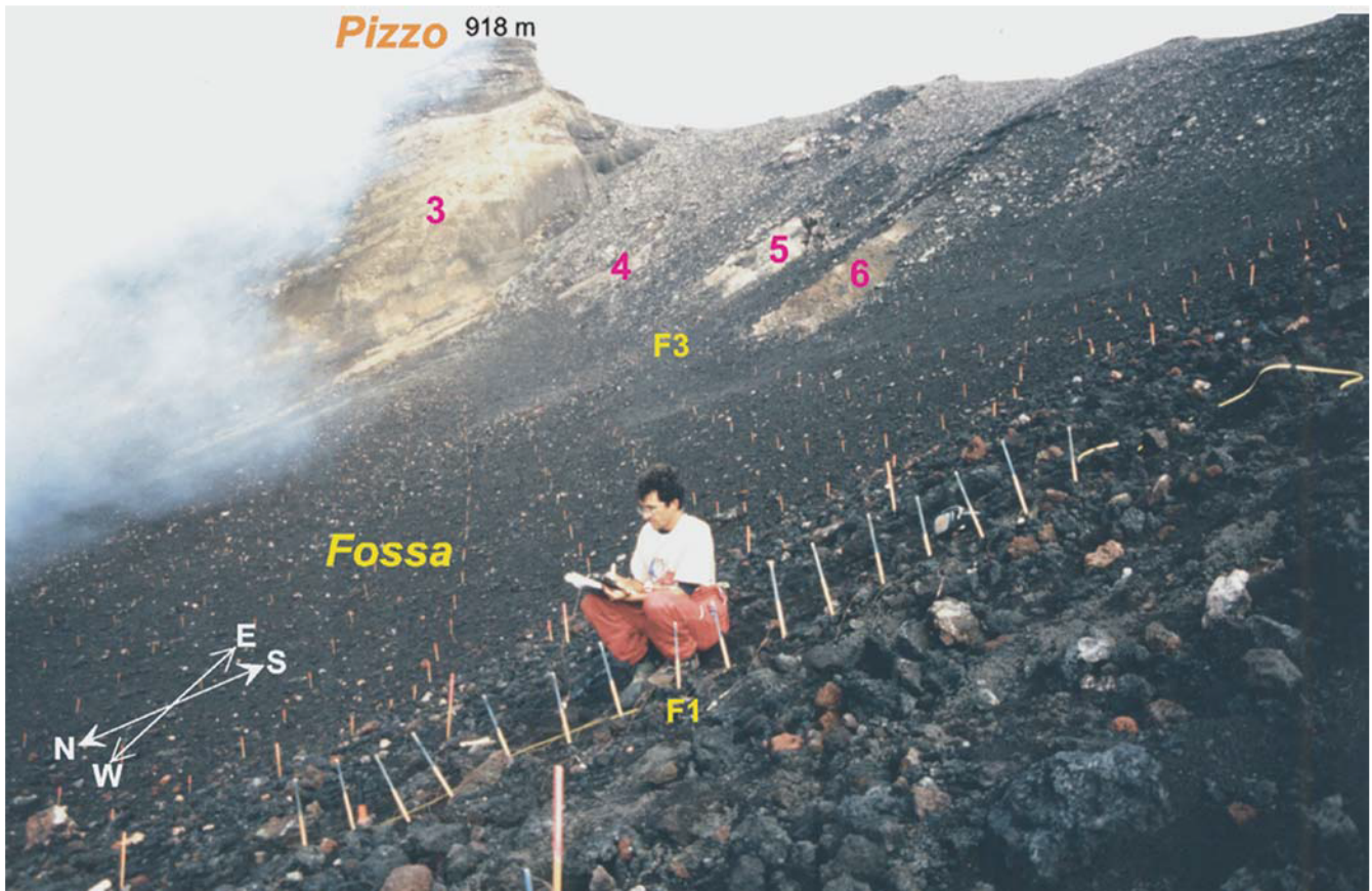
Fig. 3 Photograph showing the topographic techniques used during the field campaign with benchmarks (wooden markers) spaced 5 m apart in plan view. Red and blue markers correspond, respectively, to topographic reference and thermal sensors. F1 and F3 represent
