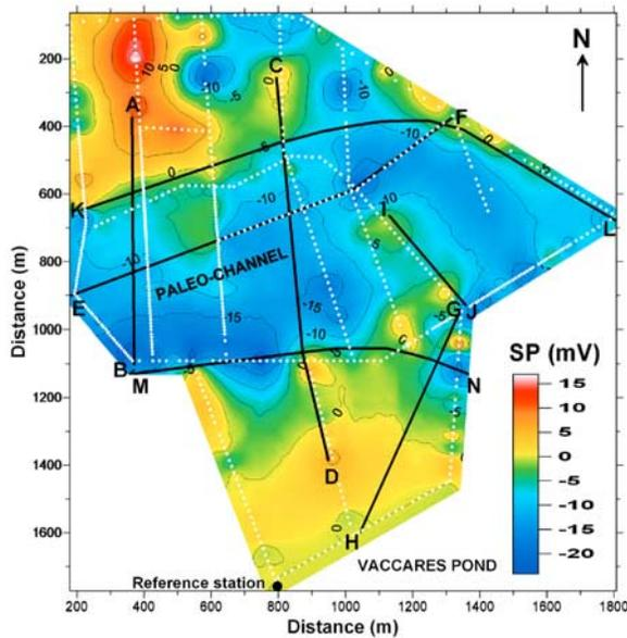
**Figure 3.** Self-potential (SP) map (in mV) with the position of the electrical resistivity profiles AB, CD, EF, GH, IJ, and GH. The fine gray line indicates the position of the SP profiles used to map the SP anomaly (the reference is located at the South of the map).
