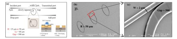
Fig.2. (a) Representation and details of single microRing and single microRaceTrack. (b) SEM images of the <u>TLR</u> device and (c) the fabrication quality on the coupling zone of one of its MR.
