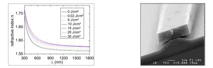
Fig. 1. Ellipsometric dispersion curves ascribed to the optical refractive index values of UV210 thin films with different deep-UV irradiation doses; scanning electron microscopy (SEM) image of a UV210 pedestal rib-waveguide.
