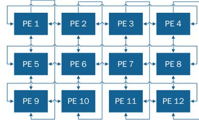
Fig. 4.  $3 \times 4$  CGRA with mesh torus topology
