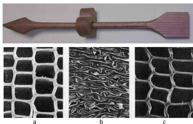
**Figure 5:** Cupido's arrow (up) and SEM images of the microstructure (down): (a) uncompressed wood; (b) heavily compressed; (c) after reconditioning (from Inoue 1982).
