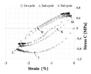
**Figure 7:** Stress of fully restrained specimen versus the unloaded strain of a specimen subjected to the same wetting-drying cycles (25°C, 30-80-30%RH): (square) 1st cycle, (triangle) 2nd cycle, (x) 3rd cycle. 0H: compression set; 0K dimensional loss for restrained or partially restrained specimens. J: stress peak, L: end of 1st adsorption; M: end of 1st cycle and start of 2nd (Mazzanti et al 2015)
