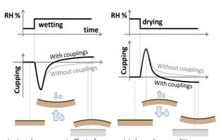
Figure 4: Transient and permanent effect of asymmetric boundary conditions.
