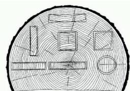
Figure 2: Deformation of wooden blocks resulting from T shrinkage exceeding R shrinkage.
