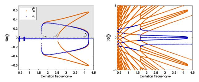
**Fig. 3.** Eigenvalues of H as a function of the excitation frequency  $\omega$ , corresponding to the simulation of Fig. 1. ' $\bullet$ ': all  $\mathbb{S}_n^k$ , for n=1,2 and  $k=0,\pm 1,\ldots,\pm H$ ; ' $\circ$ ':  $\alpha_n$ , n=1,2 computed with the Hill's method. (left): real part; (right): imaginary part. Gray region corresponds to unstable periodic solutions.
