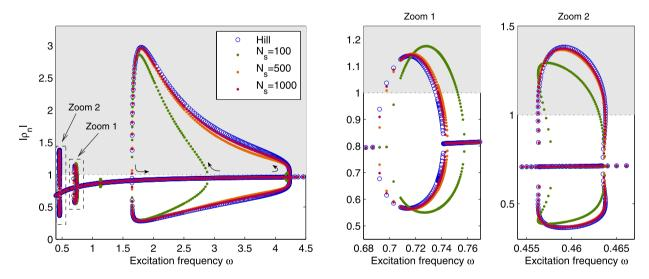
**Fig. 2.** The N=2 Floquet multipliers moduli  $|\rho_n|$  as functions of the excitation frequency  $\omega$ , corresponding to the simulation of Fig. 1. ' $\circ$ ':  $\rho_n$  computed with the Hill's method; ' $\bullet$ ':  $\rho_n$  computed with the monodromy matrix, for various numbers  $N_s$  of time samples per period T. (left): general view; (middle), (right): details of superharmonic resonance of order 2 and 3. Gray region corresponds to unstable periodic solutions.
