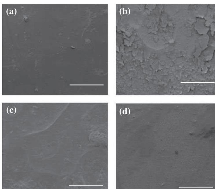
Figure 2. Scanning electron microscopic images of chitosan film without coating (a), fatty acid coating (b), beeswax coating (c), and emulsified beeswax coating (d).
