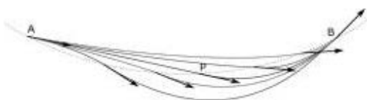
Fig. 10 Variation of the maximal curvatures of the CAC sequences in function of the intermediary pose
