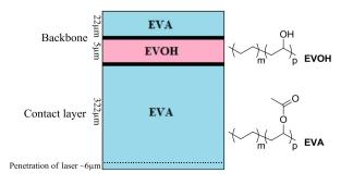
Fig. 1. Structure of film.
