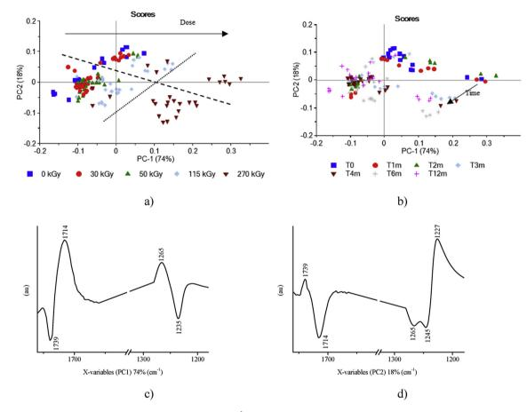
**Fig. 3.** PCA of EVA spectra at all γ-irradiation doses (1760–1670/1280–1180 cm<sup>-1</sup>). Spectra are baseline corrected and normalized. a) Score plot of PCA with γ-dose labels. Dashed line delimits the ageing groups and dotted line delimits the γ-doses groups. b) Score plot of PCA with time labels. c) Loading plot of PC1. d) Loading plot of PC2.
