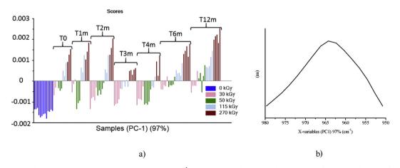
Fig. 4. PCA of EVA spectra at all γ-irradiation doses (980–950 cm<sup>-1</sup>). Spectra are baseline corrected. a) Score plot of PCA. b) Loading plot of PC1.
