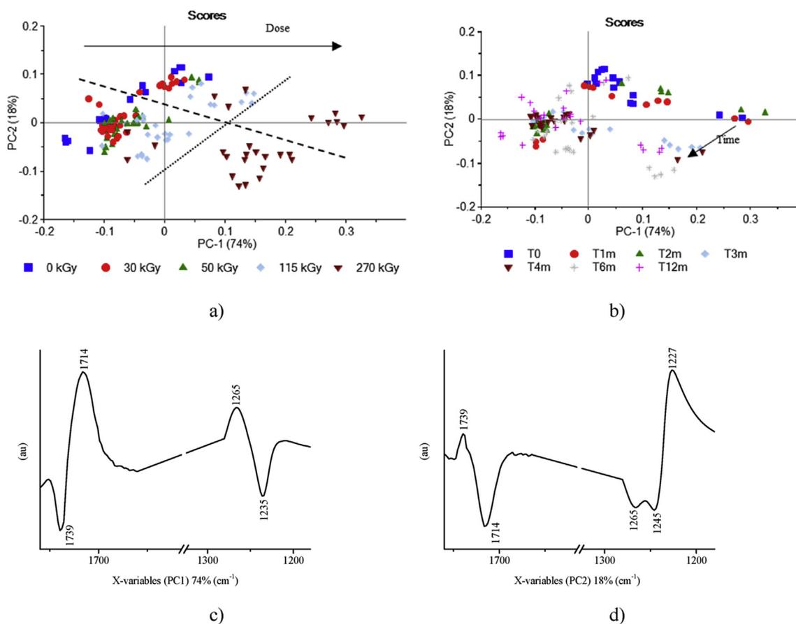
**Fig. 3.** PCA of EVA spectra at all  $\gamma$ -irradiation doses (1760–1670/1280–1180  $\text{cm}^{-1}$ ). Spectra are baseline corrected and normalized. a) Score plot of PCA with  $\gamma$ -dose labels. Dashed line delimits the ageing groups and dotted line delimits the  $\gamma$ -doses groups. b) Score plot of PCA with time labels. c) Loading plot of PC1. d) Loading plot of PC2.
