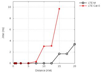
Fig. 7. Jitter variation with Distance
