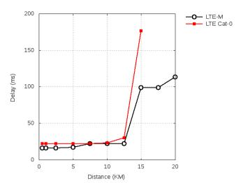
Fig. 6. Delay variation with Distance
