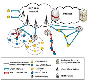
Fig. 1. LTE/LTE-M Network Architecture
