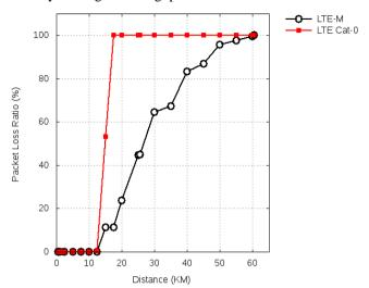
Fig. 4. Packet Loss Ratio variation with Distance
