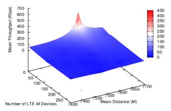
Fig. 10. Mean Throughput variation with Distance
