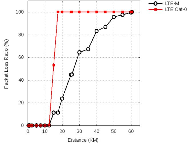
Fig. 4. Packet Loss Ratio variation with Distance
