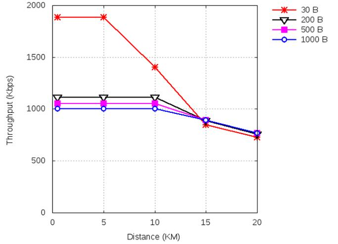
Fig. 8. Throughput and payload variation with Distance
