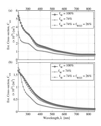
**Figure 2.** Spectral evolution of the extinction coefficient  $C_{ext}$  of spherical particles of (a) D = 29nm, (b) D = 65nm and of various compositions: pure tungsten, tungsten with spherical vacuum inclusions ( $f_W = 74\%$ ), tungsten with tungsten oxide spherical inclusions ( $f_W = 74\%$ ,  $f_{WO3} = 26\%$ ).
