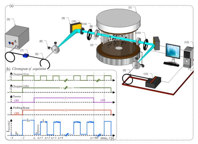
Figure A1. a) Schematic of the LES acquisition system: (1) tungsten cathode, (2) stainless-steal grounded anode, (3) glass half cylinders, (4) UV fused silica windows, (5) highly-stabilized Halogen-Deuterium lamp, (6) optical fibers, (7) on-line intensity attenuator, (8) achromatic coupling and collimating optics, (9) parabolic mirrors, (10) diaphragm, (11a - 11b) optical choppers, (12) UV-NIR spectrometer, (13) PC. b) Acquisition chronogram of the intensities
