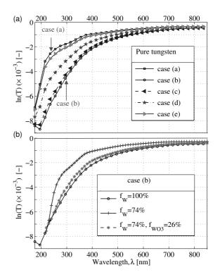
Figure 3. a) Evolution of the logarithm of synthetic transmittance spectra calculated for tugnsten spherical particles. The associated PSD parameters are reported in Table 1. b) Evolution of synthetic ln(T) spectra calculated in the case of an unimodal population (case (b) in Table 1) for pure, porous or oxidized tungsten NPs.
