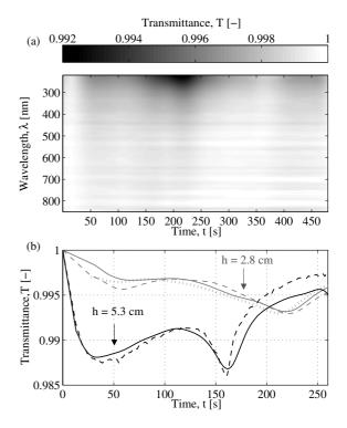
Figure 8. a) Evolution of the transmitance at different wavelengths as a function of time, 2.8 cm above the anode for a 500 s discharge. b) Transmittance at 250 nm at different heights above the anode: gray lines, h = 2.8 cm; black lines, h = 5.3 cm. Each plain, dashed, or dotted line corresponds to a separate experiment.
