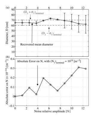
**Figure 4.** (a) Evolution of the recovered first two moments of the PSDs as a function of the relative noise amplitude. (b) Evolution of the absolute error on N as a function of the relative noise amplitude. Synthetic spectra are calculated using the PSD of case (b) (see Table 1).
