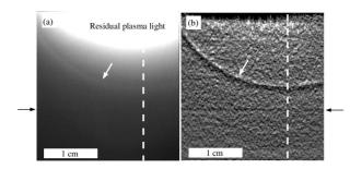
Figure 6. Typical snapshot of the scattered laser-light 45 s after plasma ignition : a) raw image, b) same as a) with an edge detection filter applied to the image. The horizontal black arrow shows the position of the lower edge of the laser sheet which was positioned 2 cm below the cathode. The oblique white arrow shows the top edge of the NP cloud. The dashed vertical line indicates the position of the discharge axis.
