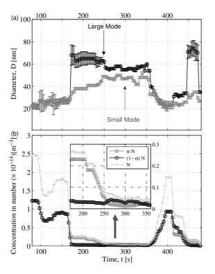
Figure 9. a) Temporal evolution of mean diameters (represented by squares or by circles) and the associated standard-deviations (represented by bars) measured by LES at the height h = 2.8 cm from the anode. A bimodal PSD is detected, its large mode is represented by the circle line, while its small mode is represented by the square line. b) Temporal evolution of N, as well as  $\alpha N$  and  $(1 - \alpha)N$  associated with the small and large modes of the PSD, respectively.
