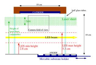
**Figure 1.** (Colour online) Schematic of the experimental set-up. The vertical position of the center of the laser-light sheet can be adjust between 1 cm and 9 cm above the anode. The field of view of the camera is adjusted to the laser-light sheet position. Note that the LES diagnostics and the laser-light scattering imaging were not implemented simultaneously.
