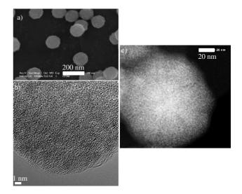
**Figure 5.** Images of a NP collected after a 300 s plasma. a) SEM. b) HR-TEM. c)HAADF-STEM. The fringe patterns in b) are the crystallites. The white dots in c) are the tungsten crystallites.
