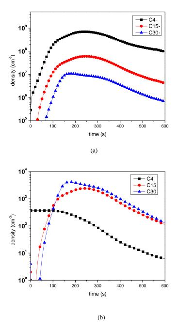
Figure 4: Time evolutions of the  $C_4$ ,  $C_{15}$  and  $C_{30}$  negative cluster densities (a) and  $C_4$ ,  $C_{15}$  and  $C_{30}$  neutral cluster densities (b) at the field reversal position, i.e., x=2.3 cm.
