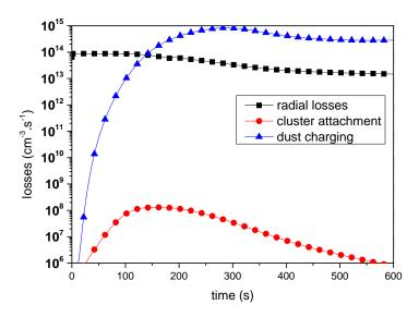
Figure 10: Time evolutions of the electron loss rates at the field reversal position, i.e., x=2.3 cm, by electron attachment to carbon clusters, electron diffusion to the reactor wall and electron losses by dust particle charging.
