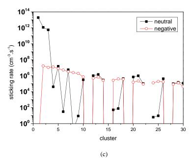
Figure 8: Contribution of the different mechanisms involved in the particle aerosol dynamics (a) time variations of the solid particle nucleation and coagulation rate at the field reversal position, i.e., x=2.3 cm, (b) the number of carbon gained per solid particle and unit time through sticking of carbon cluster at the particle surface and coagulation between solid particle and (c) contributions of the different clusters to the growth of solid particle.
