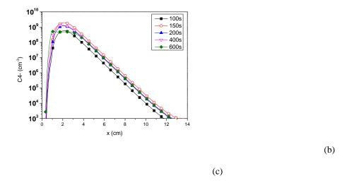
Figure 11 : Axial distributions of the  $C_4^-$  negative clusters for five time periods : 100, 150, 200, 400 and 600 s
