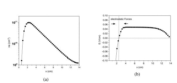
Figure 3: Axial distribution of the cold electron density (a) and the electric field (b) in the gap region for the pristine argon discharge. The cathode is located at 0 cm while the anode is at 14 cm. These profiles represent the initial distribution, the distribution at t=0 sec, for the dusty plasma model. Since the discharge is a short discharge, there is no positive column and the field remains positive beyond the field reversal position, i.e., x=2.3 cm.
