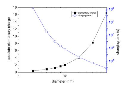
Figure 1 : Absolute elementary charge and charging time derived from the OML theory as functions of the particle diameter for Te=0.1 eV,  $n_i$ = $n_e$ = $10^{10}$  cm<sup>-3</sup>, Tg=300 K,
