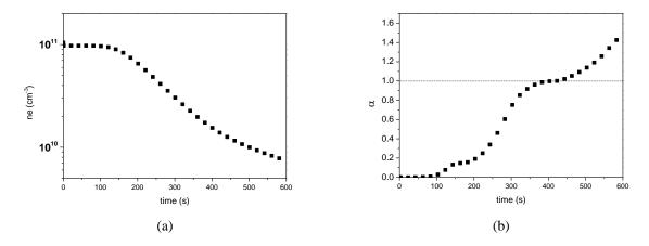
Figure 9 : Time evolutions of the electron density (a) and electronegativity factor  $\alpha$  (b) at the field reversal position, i.e., x=2.3 cm
