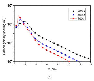
Figure 18: Axial distributions of the number of carbon gained per dust particle by coagulation (a) and through surface deposition of carbon clusters (b).
