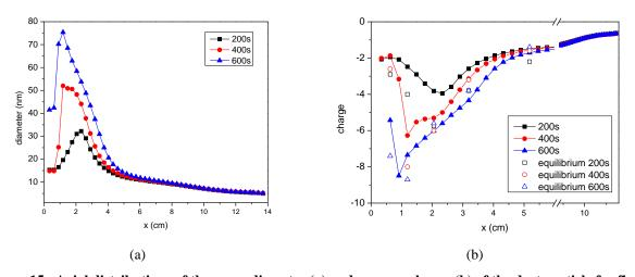
Figure 15: Axial distributions of the mean diameter (a) and average charge (b) of the dust particle for five time periods: 100, 150, 200, 400 and 600 s. The charge value obtained from OML theory are also shown (open symbols)
