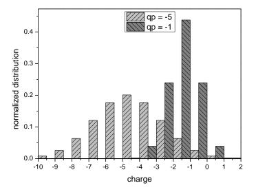
Figure 2 : charge distribution for a 5 nm particle and an average charge of -5 and -1 for Te=0.1 eV,  $n_e=n_i=10^{10}~cm^{-3},\,T_i=T_g=300~K$
