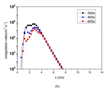
Figure 17: Axial distributions of the rate of change in dust density through nucleation (a) and coagulation (b)
