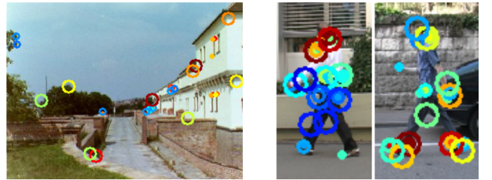
Fig. 2. Junctions shown by circles for one landscape image and two pedestrian images. The radius corresponds to the scale, and the colour to the absolute value of junction-ness (the red corresponding to the highest values).
